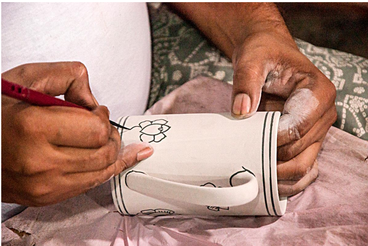
Floral motifs are drawn on the articles with oxide color solution.
